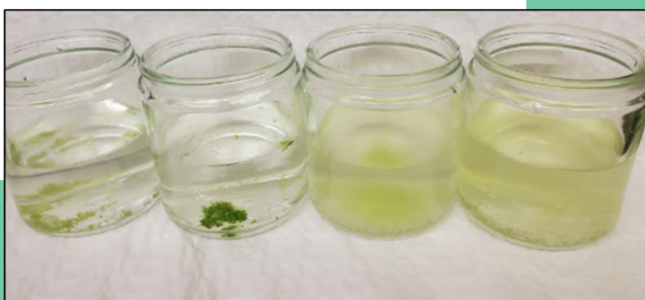
Figure 2. Precipitated algae flocs formed from (left to right) BioFlow + chitosan flakes; BioFlow + GeoFlow; chitosan powder + modified bentonite clay; and chitosan flakes + modified bentonite clay.
