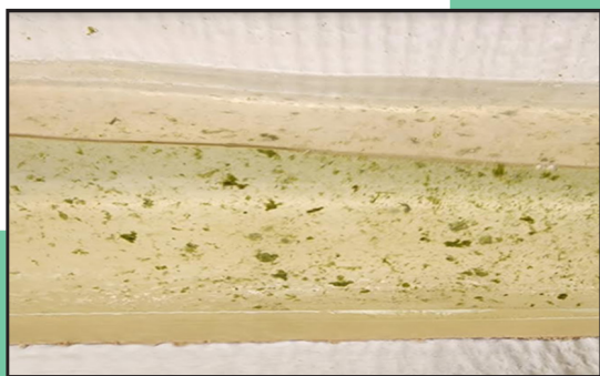
Figure 4. Algae flocs in wave tank formed by BioFlow + chitosan flakes.
