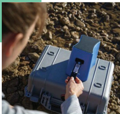
Figure 2. Anticipated final product of a SHA-based sensor cartridge that can produce readout in a portable MBio® LightDeck™ diagnostic platform (collaborative work with BGSU).
