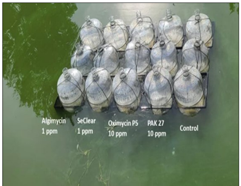
Figure 2: Tested mesocosm setup at the western basin of Lake Erie
