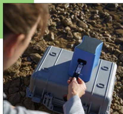
Figure 2: The anticipated final product of a sandwich hybridization assay (SHA)-based sensor cartridge that can produce readout in a portable MBio® LightDeck™ diagnostic platform (collaborative work with BGSU)
