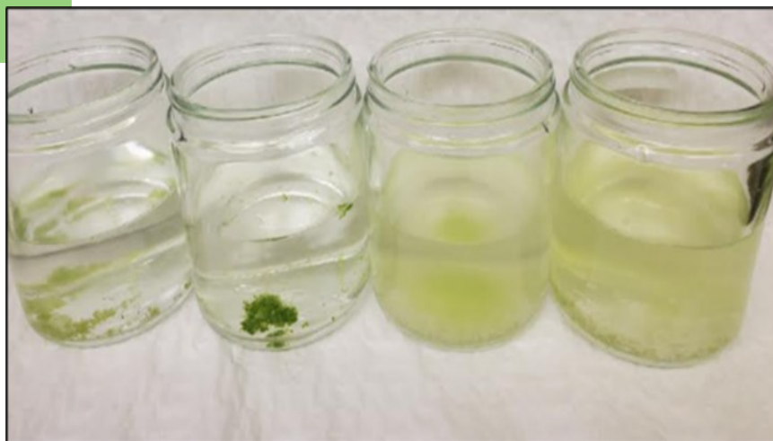
Figure 2: Precipitated algae flocs formed from (left to right) BioFlow and chitosan flakes, BioFlow and GeoFlow, chitosan powder and modified bentonite clay, and chitosan flakes and modified bentonite clay.
