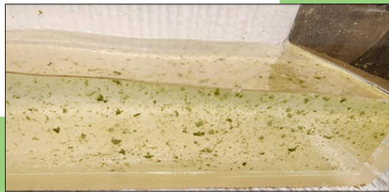
Figure 4: Suspended algae flocs in wave tank formed by BioFlow and chitosan flakes. The wave motion within the tank yielded slower flocculation and precipitation rates compared to vortex mixing.
