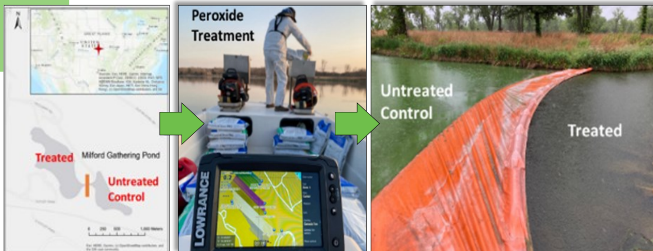
Figure 4: Initial field-scale demonstrations (Milford Gathering Pond, KS) treating overwintering cells in sediments indicate decreased severity of HAB. The map depicts the treated and untreated (control) areas of the lake. The images show researchers administering treatment and the subsequent results.
