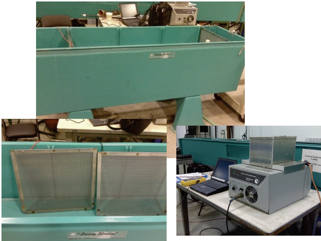
Figure 4. Exposure tank, electrodes, and power supply employed in the electrical exposures.
