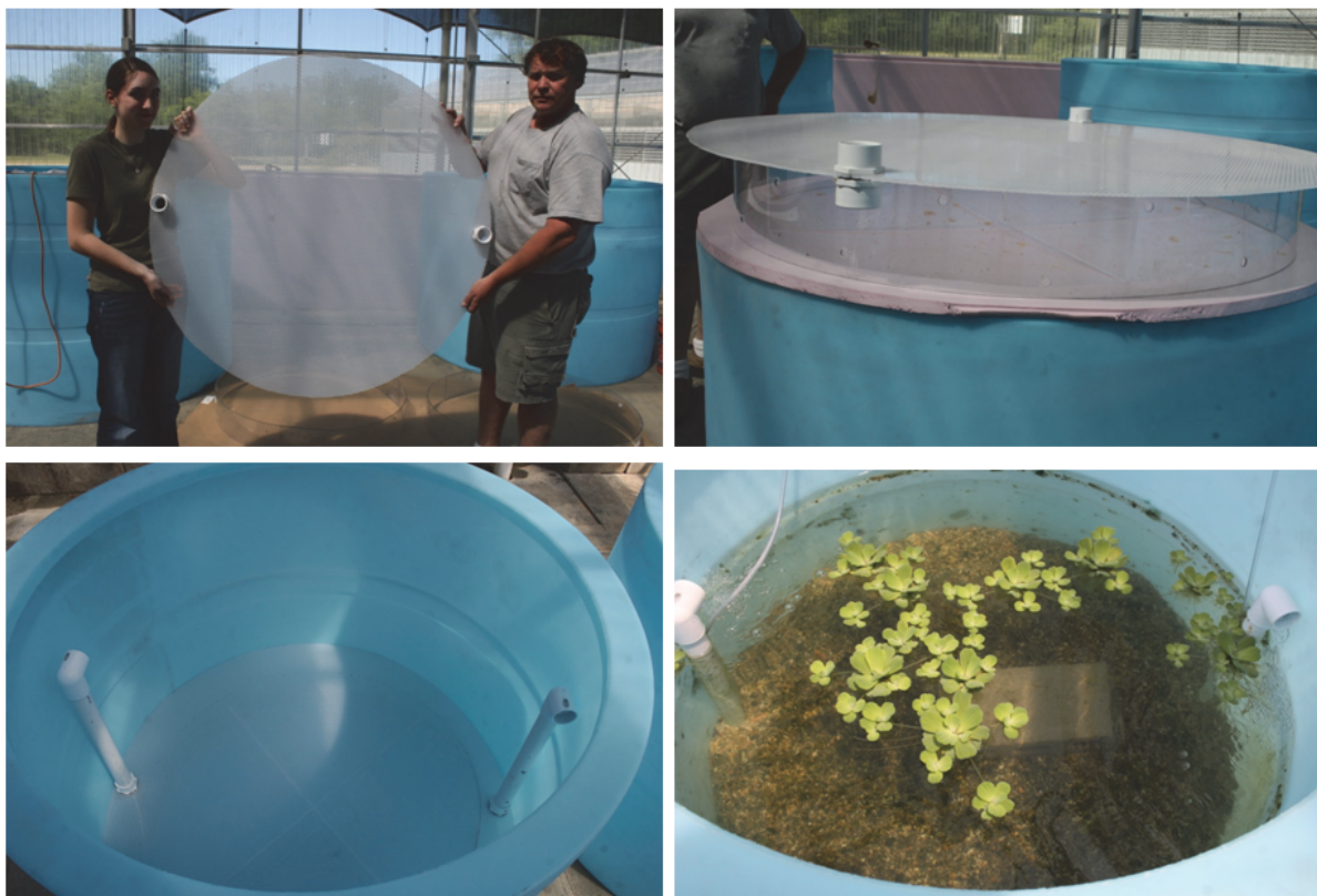
Figure 3. Mesocosm construction (clockwise from upper left): polypropylene disc with staggered holes 5 mm in diameter and two fittings for PVC pipe; base of undergravel filter formed by disc placed on plastic rim surrounding Plexiglas cross-piece (pink pad is used as insulation under the tank); bird's eye view of undergravel filter with lift tubes in place; bird's eye view of assembled mesocosm with gravel, cinder block, and plants in place and water circulating.
