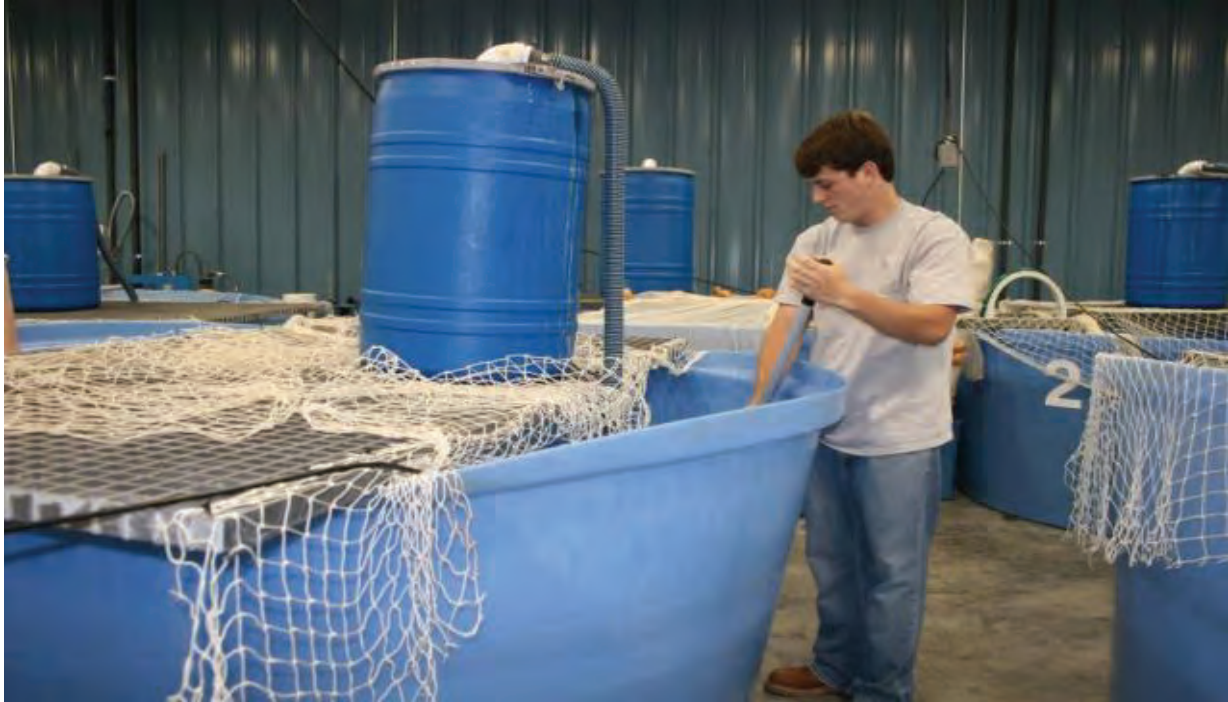
Figure 2. Holding tanks used to maintain bighead carp and silver carp in the laboratory. Water is pumped by submerged pumps into overhead filters supported on fiberglass grids. Water passes through ammonia-removing resin chips, carbon, and foam pads and then showers back into the tank. Net skirts attached to grids prevent silver carp from jumping out of the tanks.
