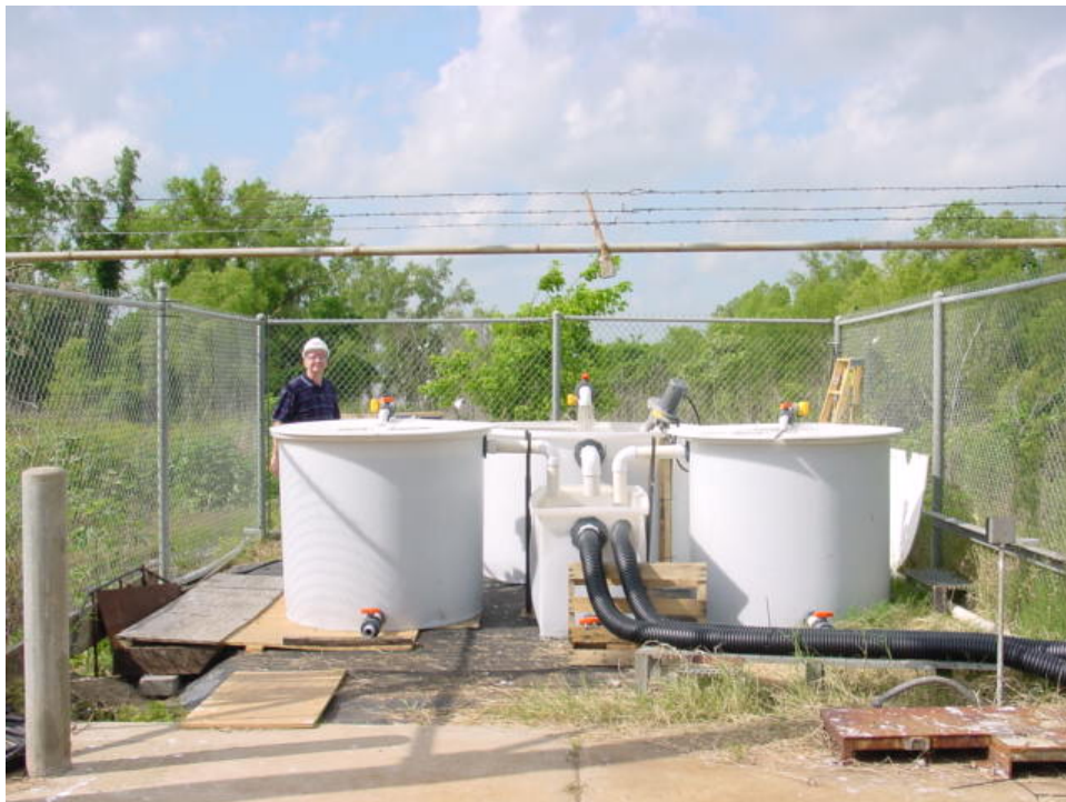
Figure 4. Trial set up on the Mississippi River near LaPlace, LA. Tank 1 is the collection tank in the back center and contains the filter box. Tank 2, on the left, receives the filtered water. Tank 3, on the right, is the control tank receiving unfiltered water from the Mississippi River
