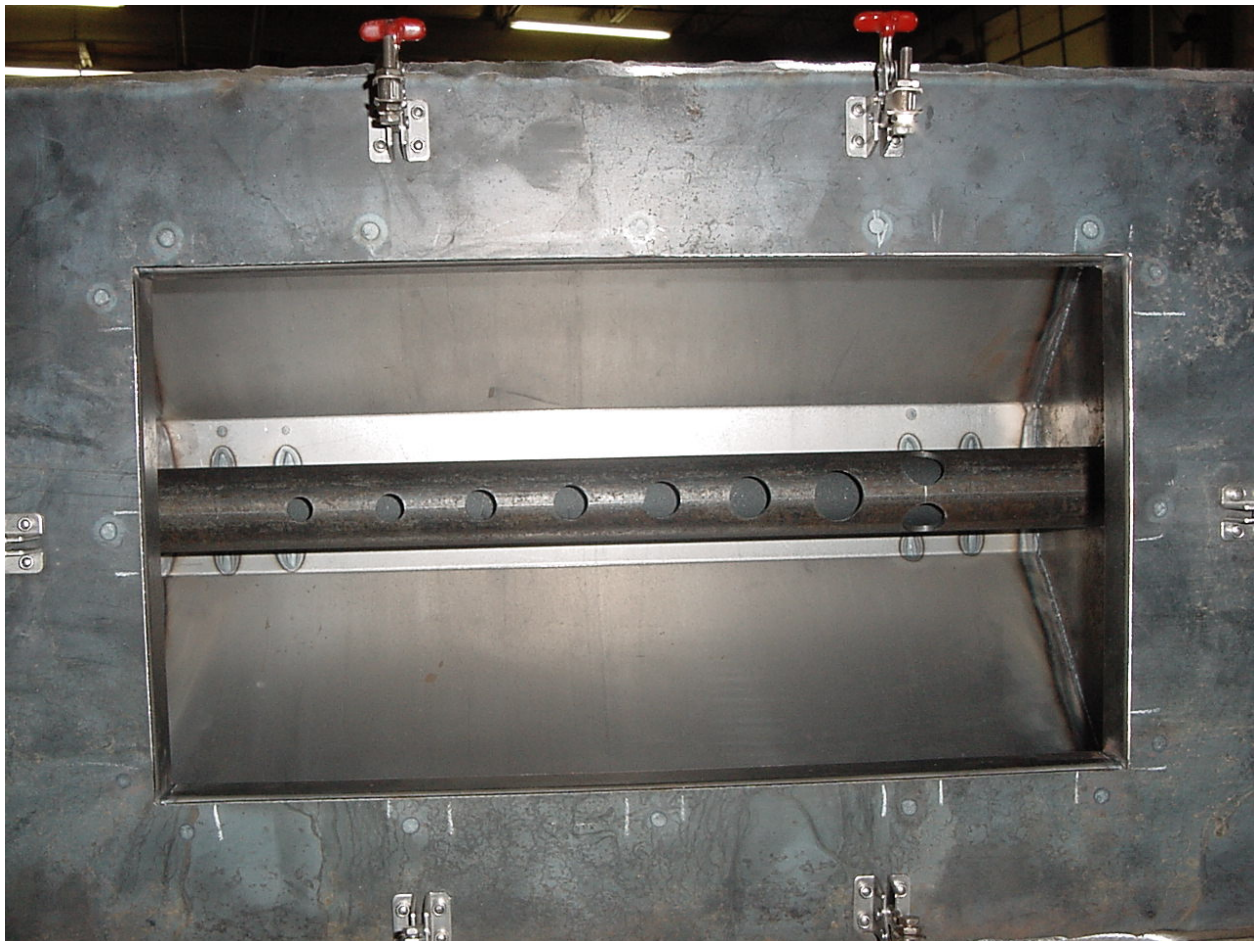
Figure 1. PCI's patented flow control device inside the filter boxes draws water uniformly across the face of the pleated filter(s)
