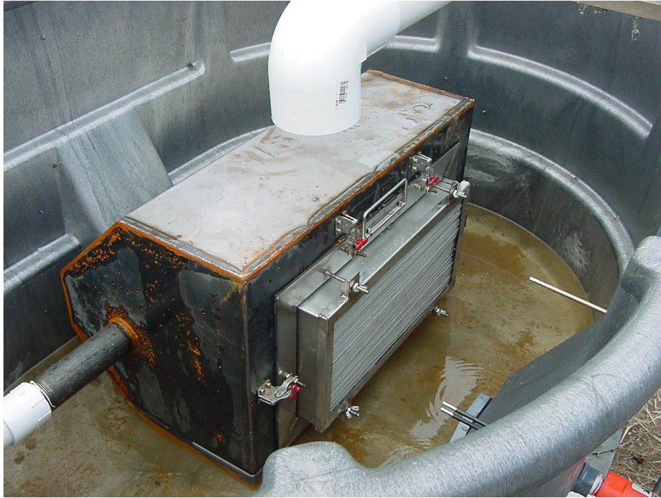
Figure 3. Filter box set inside tank for trials on Lake Ontario site. The filter face was 8 by 16 in. (0.2 by 0.4 m) with 3.5-in.- (0.09-m-) deep pleats. A pleated pre-screen measuring 8 by 16 by 2 in. (0.2 by 0.4 by 0.05 m) deep was also used
